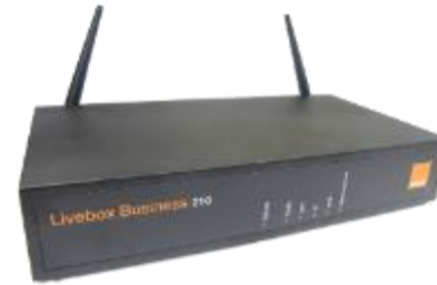
Box build assembly of voice & data routers for enterprises VT Automotive Electronics
