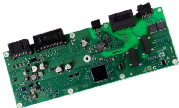
Battery management unit VT Automotive Electronics
