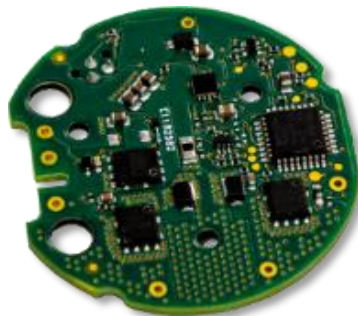
Oil pump controller VT Automotive Electronics
